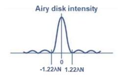
Rayleigh criterion for  $\lambda = 10 \mu m$  N = f/1.0  $R_{Airy\ Disk} \approx 1.22 \times \lambda \times N$  $\approx 12 \mu m$
