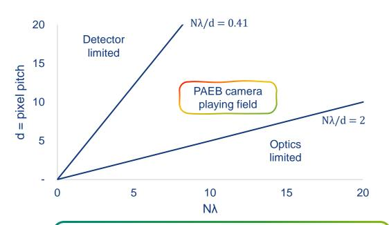
A balanced design of sensor and optics makes an affordable thermal camera possible as part of a PAEB sensor system.
