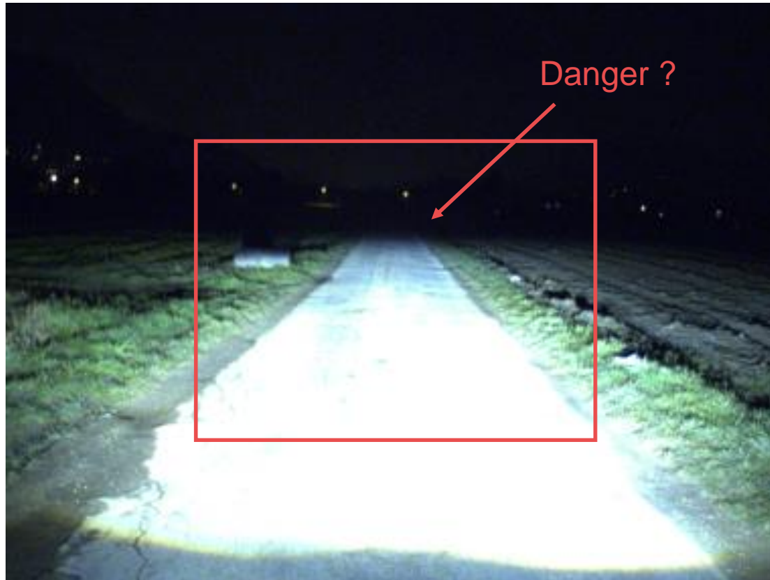
Xenon low-beam according to ECE-R98
